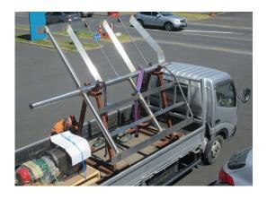
Large gate, or anchor, mixer for 15 cubic meter vessel processing chocolate. Photo shows it loaded on truck to get polished by professional metal polishes before installation in vessel.
