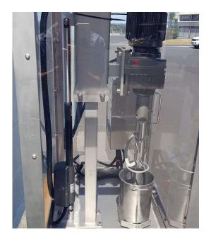
The enclosure has an industrial safety door switch to prevent the mixer from operating with the door open. The complete mixer assembly raises and lowers by means of a motorized linear actuator operated from the control panel.
