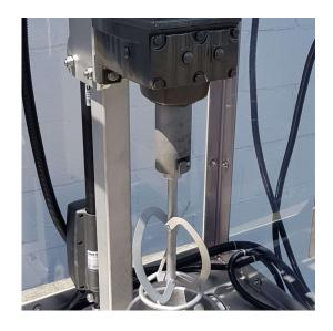
Our engineering team studied the application and considered the customer requirements to design both an effective mixer and fully self contained safe solution. The mixer shaft and impeller is held in position and driven by a bayonet type shaft coupling allowing the quick removal of the shaft without the use of tools.
