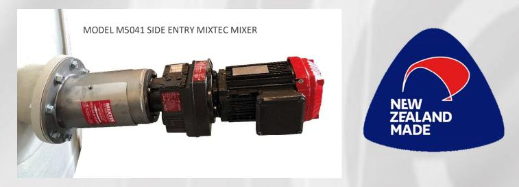
**Mixtec 5041 Side Entry Mixers WITH EXTERNAL SHUT OFF DEVICE:** Specifically designed for the wine industry, this cost effective and energy efficient mixer is fitted with our low shear Mixtec HA700 hydrofoil impeller ensuring maximum flow rates using minimum motor power. A compact design with stainless steel angled mounting stool and curved face mounting flange allows for simple installation and ensures the correct flow patterns throughout the tank.
